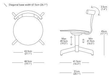
\* Components drawn in relative scale. Refer to CAD files for accurate drawings
